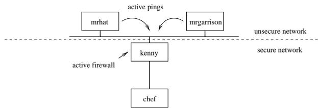
Fig. 5. **Active Firewall Experimental Set-up**
