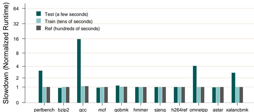
**Fig. 4.** Avoiding the performance hit during the dynamic relocation discovery phase (first run) by gradually increasing the input size on each execution. The overall time in this case is much less compared to running a program using large input the first time.
