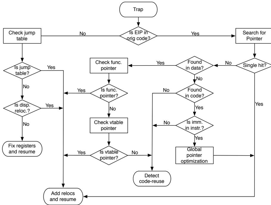
**Fig. 2.** Flow graph of the procedure followed after a memory access exception (trap) is generated. If the instruction pointer (EIP register) at the time of the exception is within the original code segment, the system performs pointer verification, otherwise the faulting instruction is fixed.
