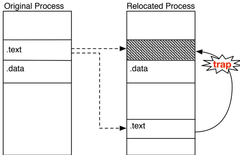
**Fig. 1.** High-level overview of runtime relocation fixup. The code segment of a stripped binary is loaded to a randomly chosen location, and its original memory area is marked as inaccessible. Memory accesses and control transfers to any of the original locations are trapped. Relocation information is then reconstructed by analyzing the faulting instruction.
